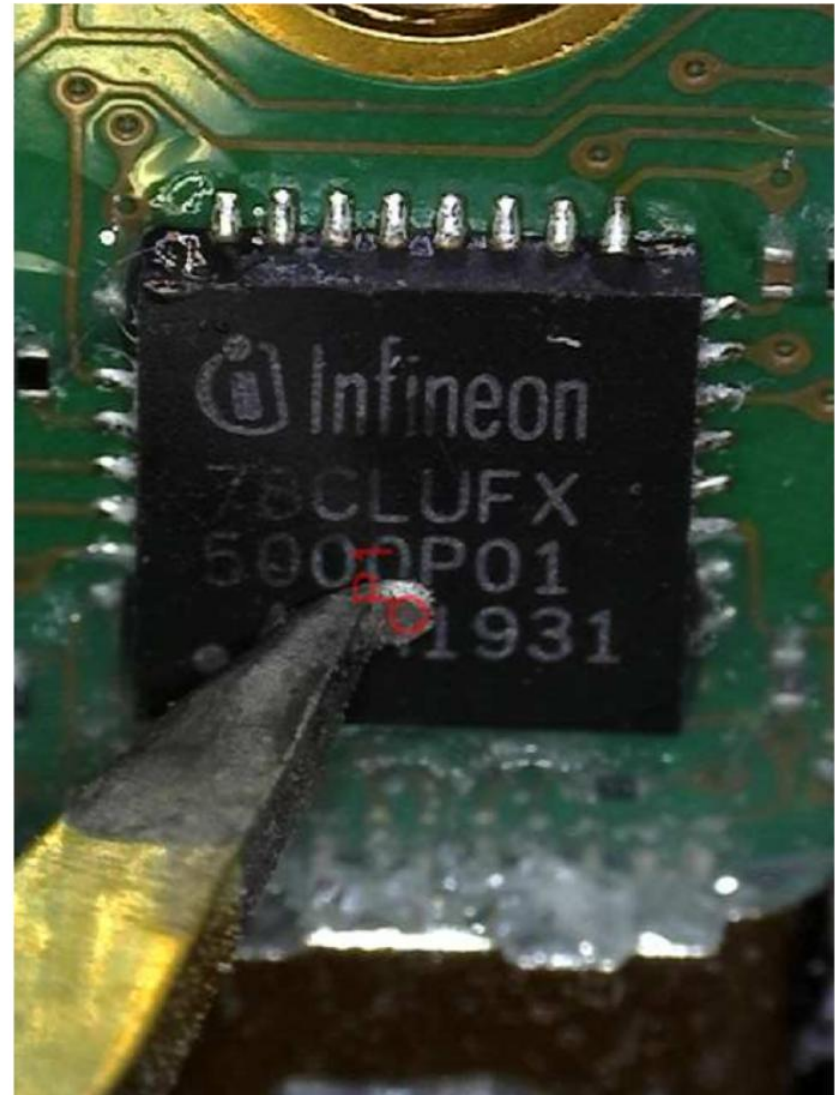
Figure 1.4: YubiKey 5Ci – EM Acquisition Setup
