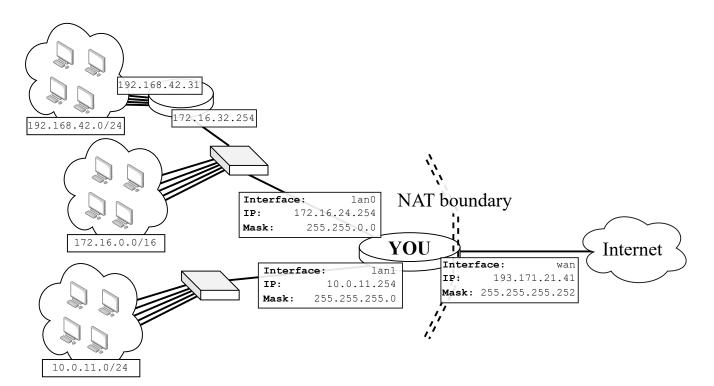
Your default gateway for any networks not listed is 193.171.21.42. Your task is to correctly route packets, and to apply NAT to allow devices to communicate with the internet.
