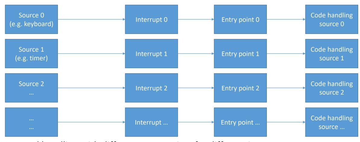
Vectored handling with different entry points for different interrupts
