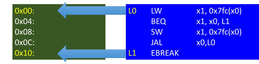
The label "L0" is a symbolic name for the memory location with address 0x00. Likewise, the label "L1" is a symbolic name for the memory location with address 0x10.
