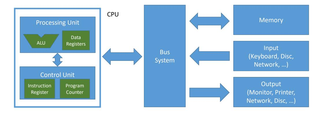
The bus system takes care of routing the load/store operations to the correct physical device as defined by the memory ranges
